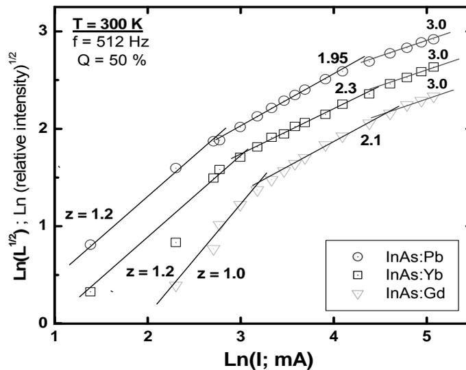
Figure 9. The relative electroluminescence intensity ( $L$ ) – current ( $I$ ) characteristics measured from the various LEDs plotted as  $\ln(L^{1/2})$  against  $\ln(I)$ : circles – InAs: Pb, squares - InAs: Yb, triangles - InAs: Gd. The slope represents the index  $z$  in the equation  $I = An+Bn^2+Cn^3$  and reveals the different recombination mechanisms operating as the current injection increases .
