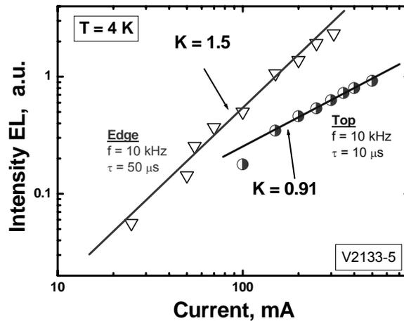
Figure 21. The light–current characteristics measured from the surface and edge of the ring geometry LED at 4K
