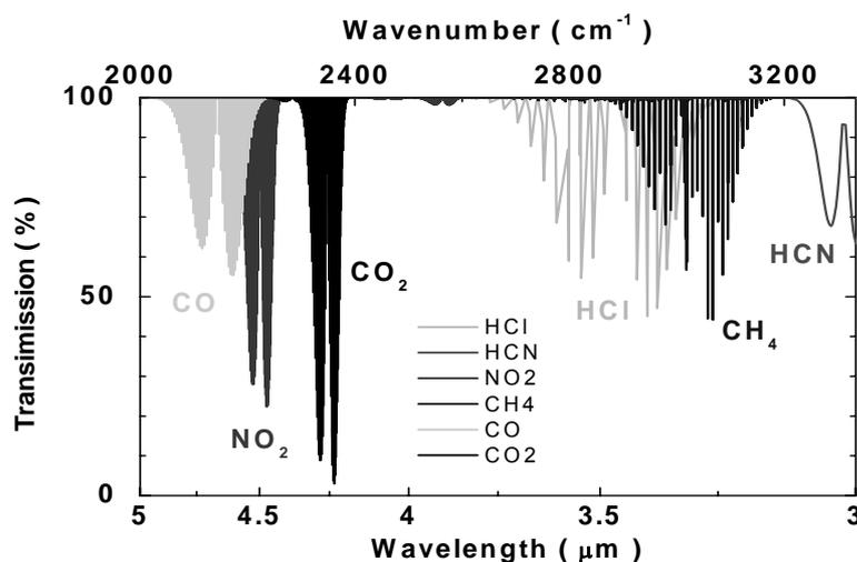
Figure 1. Some target gas absorption spectra in the mid-infrared spectral range.
