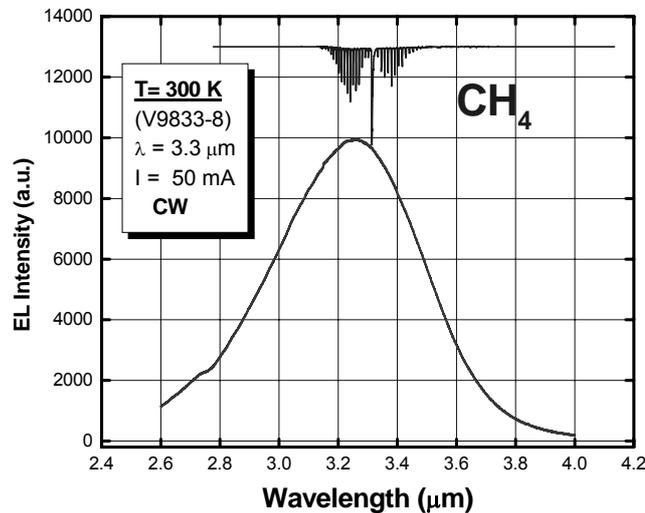
Figure 5 The electroluminescence emission spectrum of an InAs double heterostructure LED at 300 K
