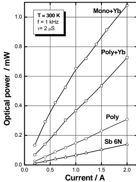
Figure 4 The optical output power characteristics measured from  $4.6 \mu\text{m}$  LEDs prepared with different purification treatments of the InAsSb active region (after Krier *et al.*)
