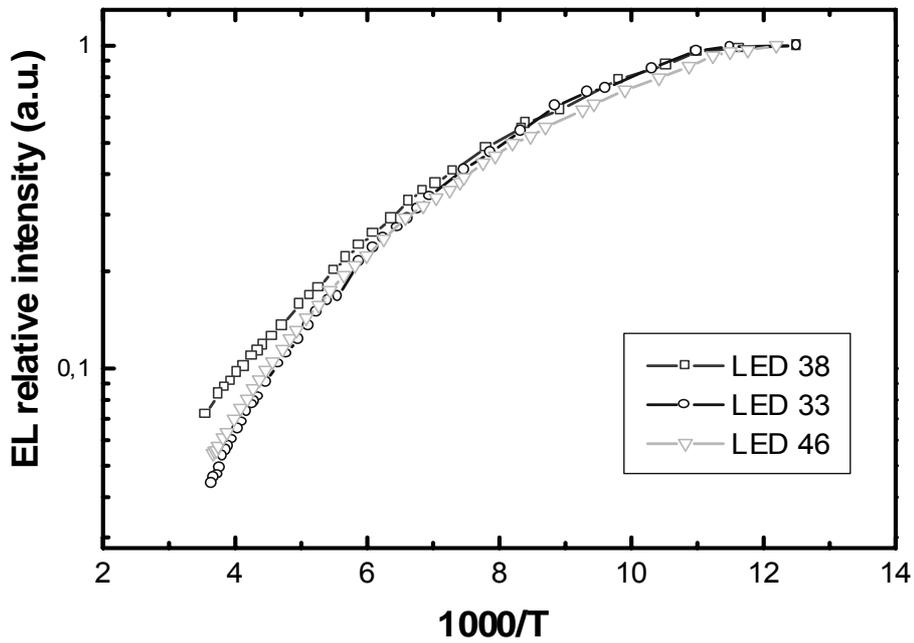
Figure 13. A comparison of the normalised temperature dependence of electroluminescence emission intensity of 3.3, 3.8 and 4.6  $\mu\text{m}$  LEDs over the temperature range 77-300 K (after Krier *et al.* )
