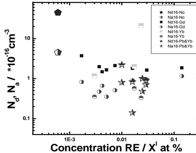
Figure 6. The dependence of residual impurity concentration on the rare earth gettering or melt purification methods used.
