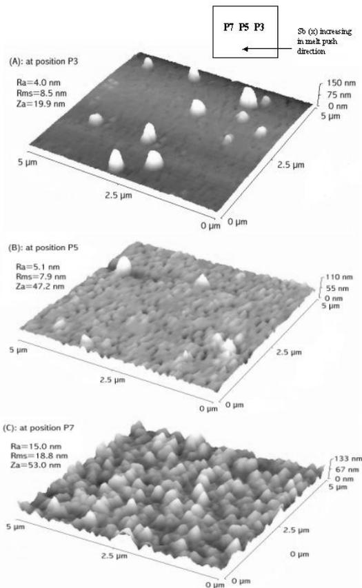
Figure 14. The AFM images obtained from un-encapsulated  $\text{InAs}_{1-x}\text{Sb}_x$  quantum dots with increasing Sb composition grown by LPE and corresponding to the passing direction of the melt across the substrate. Approximate compositions are A ( $x=0.20$ ); B ( $x=0.25$ ); and C ( $x=0.30$ ) Reprinted with permission. Copyright 2000. American Institute of Physics
