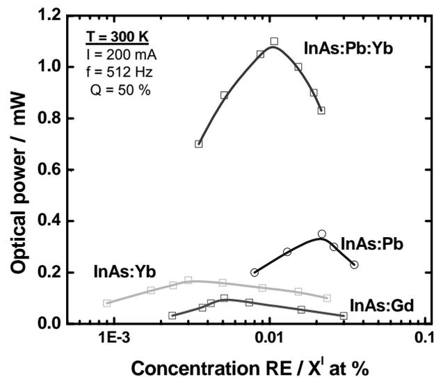
Figure 7. The dependence of the LED output power on concentration for the different purification methods used.
