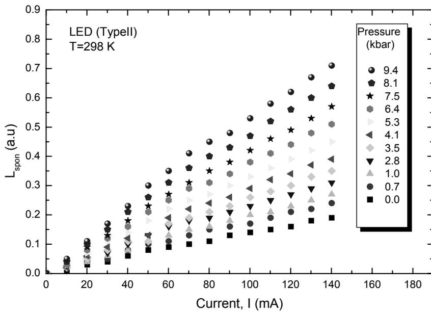
Figure 10. Measured integrated spontaneous emission intensity as a function of current for 0 kbar <math>P</math> <math>9.4</math> kbar at room temperature for an InAs/InAsSbP 3.3  $\mu\text{m}$  LED .
