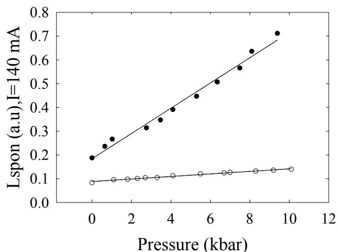
Figure 11. A comparison of the pressure dependence of the electroluminescence emission intensity for type-I (3.8  $\mu\text{m}$ , open points), and type-II (3.3  $\mu\text{m}$ , solid points) double heterostructure LEDs at 300 K. Reprinted with permission Copyright 2003 AIP<sup>76</sup>.
