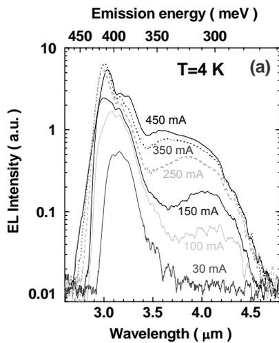
Figure 17. The 4 K EL spectrum of the QD LED at various injection currents Reprinted from A. Krier, X-L Huang, *Physica E*, **15**, 159 (2002) with permission from Elsevier
