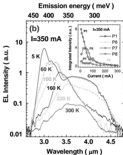
Figure 18. The integrated EL intensity dependence on temperature at 350 mA injection current. Reprinted from A. Krier, X-L Huang, *Physica E*, **15**, 159 (2002) with permission from Elsevier
