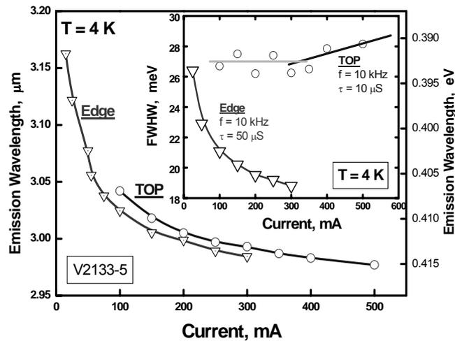
Figure 20. The current tuning behaviour of peak emission wavelength for edge and surface (Top) emission from the LED measured at 4K at a frequency of 10 kHz using 50 % duty cycle (50  $\mu\text{s}$  pulses). The inset shows the corresponding FWHM variation with current, ( duty cycle reduced to 10% at highest current to control Joule heating) .
