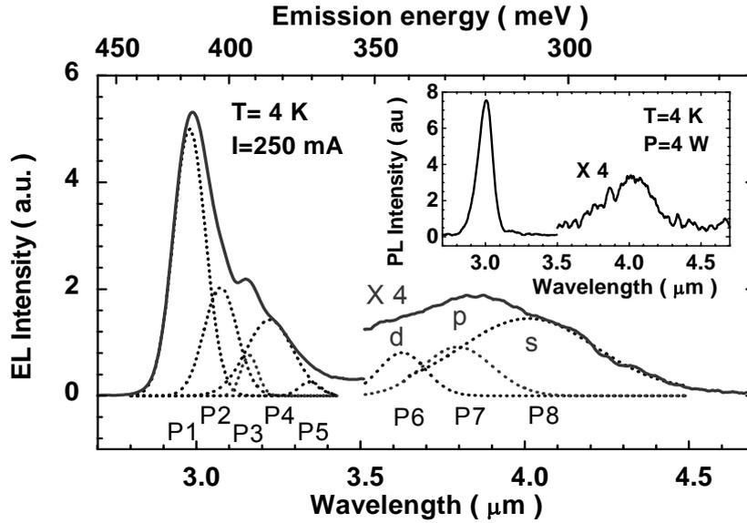
Figure 15. The electroluminescence emission spectrum obtained from an InAsSb quantum dot LED measured at 4 K using 250 mA injection current. De-convolution reveals the s,p,d confined state transitions of the QD. The inset shows the PL spectrum at 4 K for comparison. Reprinted from A. Krier, X-L Huang, *Physica E*, 15, 159 (2002) with permission from Elsevier
