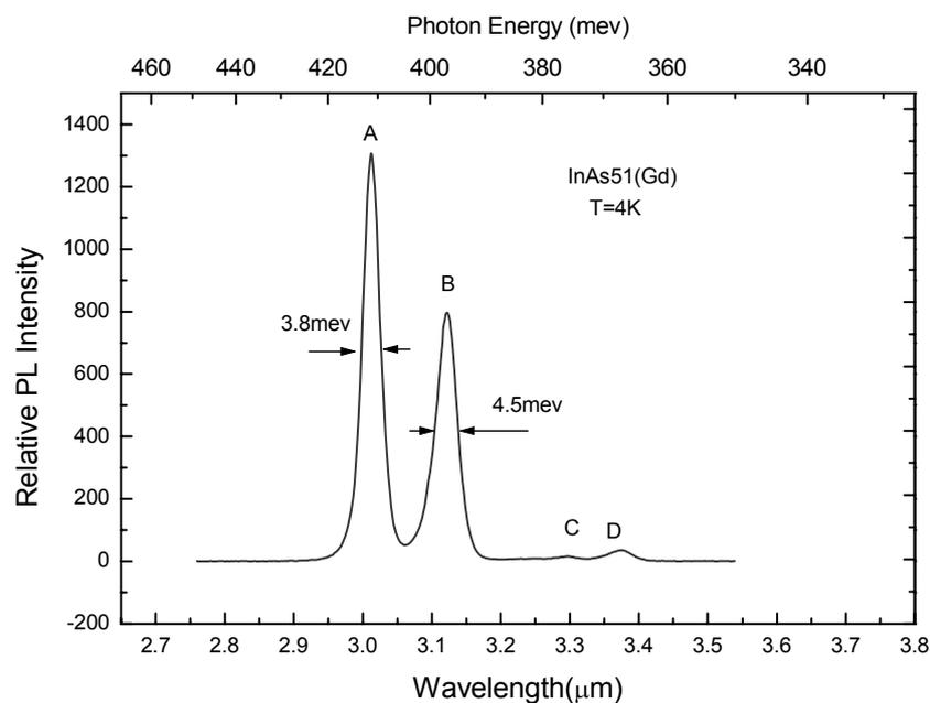
Figure 2. Low temperature photoluminescence spectrum of InAs prepared using Gd gettering of the melt during LPE growth (after Gao *et al.*<sup>60</sup>)
