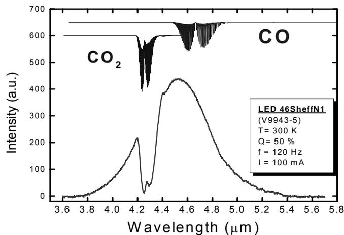
Figure 3 The electroluminescence emission spectrum of an InAs<sub>0.89</sub>Sb<sub>0.11</sub> LED at 300 K
