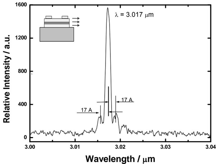
Figure 22. The mode spectrum obtained at 80 K from a mid-infrared whispering gallery mode ring laser .
