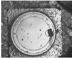
Figure 19. Nomarski microscope photograph of a typical mesa etched LED (350  $\mu\text{m}$  diameter) with ring contact electrode (30  $\mu\text{m}$  wide).
