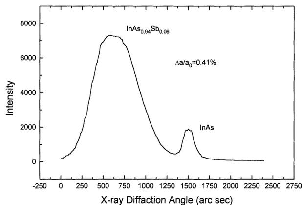
**Figure 2.** Double crystal x-ray rocking curve for a single InAs<sub>0.94</sub>Sb<sub>0.06</sub> epilayer grown on an InAs(100) substrate by LPE, which was used as the buffer layer in our structure.
