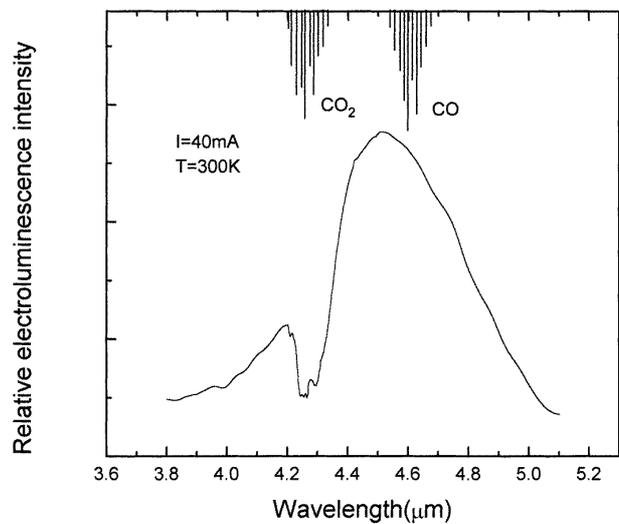
**Figure 8.** 300 K electroluminescence emission spectrum measured in the laboratory atmosphere from one of the InAsSbP/InAsSb LEDs and the corresponding fundamental  $\text{CO}_2$  and CO gas absorptions.
