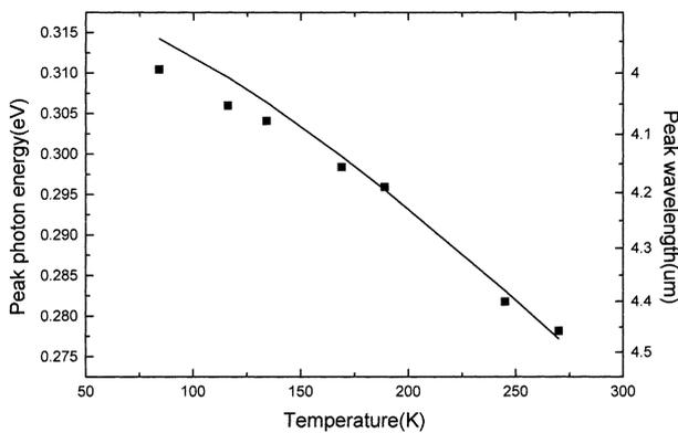
**Figure 7.** The temperature dependence of the electroluminescence peak emission energy (full squares) of one of the InAsSbP/InAsSb LEDs compared with the theoretical temperature dependence of the band gap (full curve) calculated from [23].
