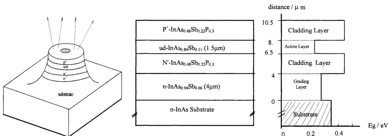
**Figure 1.** The basic device structure and the energy-band diagram of the InAsSbP/InAsSb double heterostructure LEDs showing the InAs<sub>0.94</sub>Sb<sub>0.06</sub> step mismatched buffer layer of intermediate composition.
