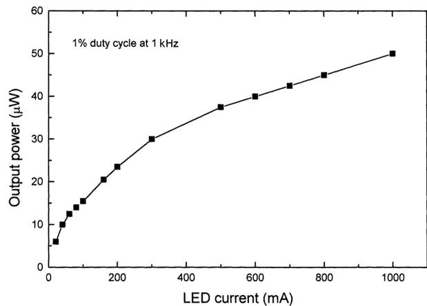
**Figure 9.** Total power output from one of the InAsSbP/InAsSb LEDs against peak pulse drive current measured using a 1% duty cycle at 1 kHz.
