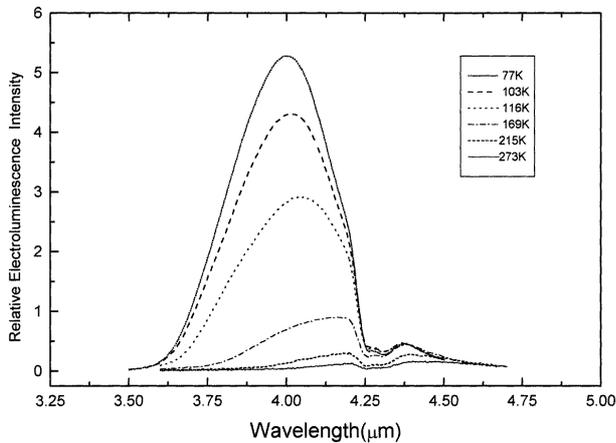
**Figure 6.** The electroluminescence emission spectra obtained from one of the LEDs measured at different temperatures from 77 K to 273 K. (40 mA peak pulse drive current, 20% duty cycle in each case.)
