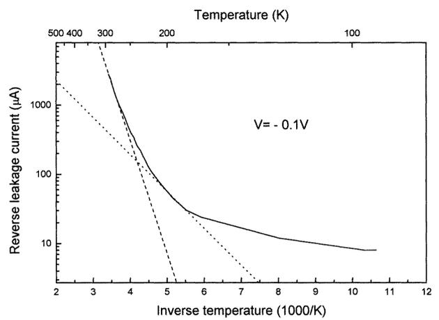
**Figure 5.** The diode reverse leakage current against an inverse temperature of one of the InAsSbP/InAsSb LEDs measured at  $-0.1$  V.
