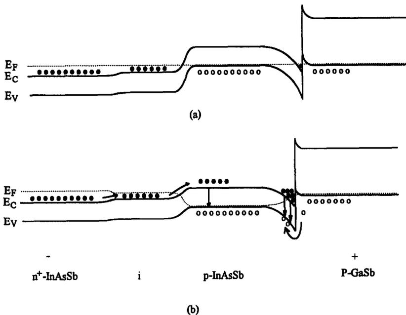
Fig. 5. The energy-band diagram of the  $n$ - $i$ - $p$ - $\text{InAs}_{0.91}\text{Sb}_{0.09}/\text{P-GaSb}$  structure. (a) Zero bias; (b) forward bias.
