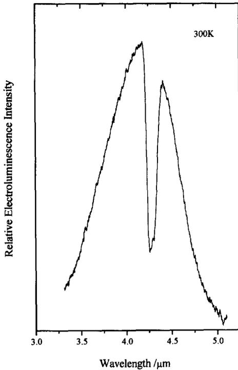
Fig. 4. Room temperature emission spectrum of an  $n$ - $i$ - $p$ - $\text{InAs}_{0.91}\text{Sb}_{0.09}/\text{P-GaSb}$  LED measured in the laboratory atmosphere.
