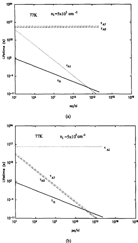
Fig. 2. Dependence of calculated carrier lifetime on normalized doping concentrations for  $\text{InAs}_{0.90}\text{Sb}_{0.91}$  at 77 K for n-type (a) and p-type (b).
