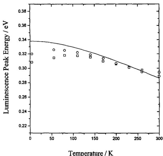
Fig. 6. Luminescence peak energy of EL and PL versus temperature. (□) EL of n-i-p-InAs<sub>0.91</sub>Sb<sub>0.09</sub>/P-GaSb; (○) PL of undoped n-type InAs<sub>0.91</sub>Sb<sub>0.09</sub>; (—) theoretically calculated temperature dependence of the energy gap for InAs<sub>0.91</sub>Sb<sub>0.09</sub> alloy.
