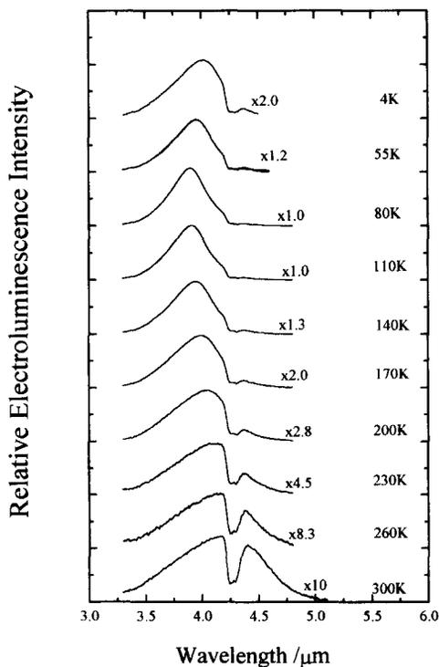
Fig. 3. The EL emission spectra measured at various temperatures for the n-i-p- $\text{InAs}_{0.91}\text{Sb}_{0.09}$ /P-GaSb LED.
