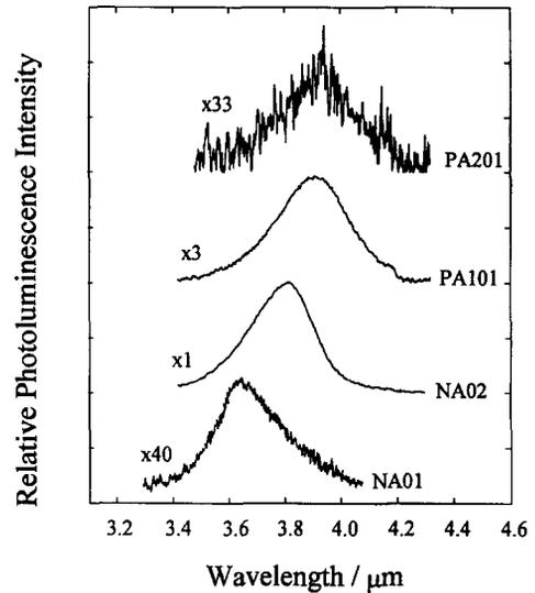
Fig. 1. The 78 K photoluminescence spectra from 4  $\mu\text{m}$  thick Te doped n-type sample (NA01), 4  $\mu\text{m}$  thick undoped n-type sample (NA02) and two 6  $\mu\text{m}$  thick zinc doped p-type samples (PA101 and PA201).
