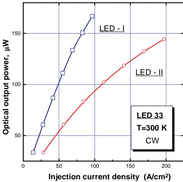
**Figure 5.** Light-current characteristics measured from the LEDs prepared with different contact geometries. LED I is  $450 \times 450 \mu\text{m}^2$  square with a ring contact  $300 \mu\text{m}$  in diameter and a Yb purified active region, LED II is a mesa-etched LED chip with a diameter of  $300 \mu\text{m}$ . The characteristics were measured at room temperature using a 50% duty cycle at 430 Hz.
