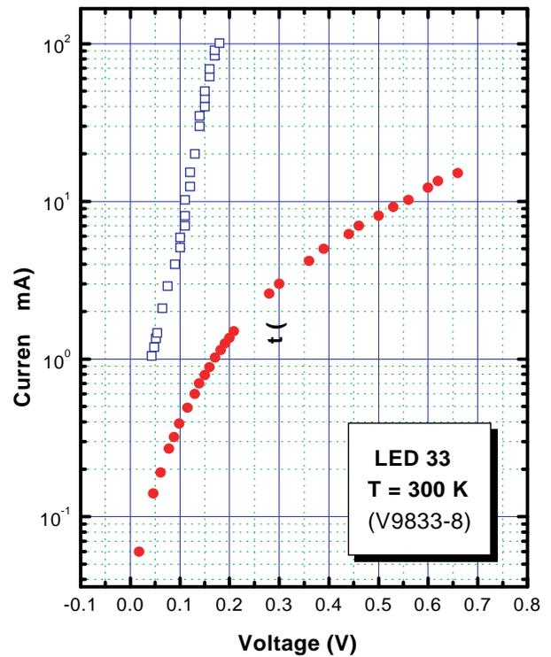
**Figure 3.** A semi-logarithmic plot of a typical current–voltage characteristic for one of the square LED chips (LED I) measured at room temperature.
