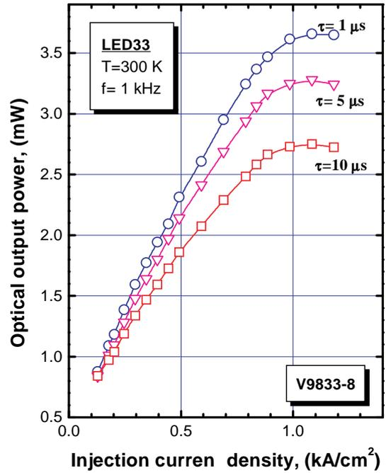
**Figure 6.** Light-current characteristics measured from LED I. The characteristics were measured at room temperature at a drive current of 1 kHz using 0.1%, 0.5% and 1% duty cycles with  $1 \mu\text{s}$ ,  $5 \mu\text{s}$  and  $10 \mu\text{s}$  pulses, respectively.
