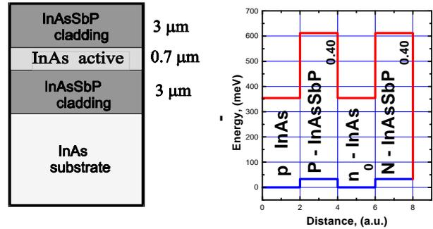
**Figure 1.** The basic device structure and the energy-band diagram of the InAsSbP/InAs/InAsSbP double heterostructure LEDs grown by LPE.
