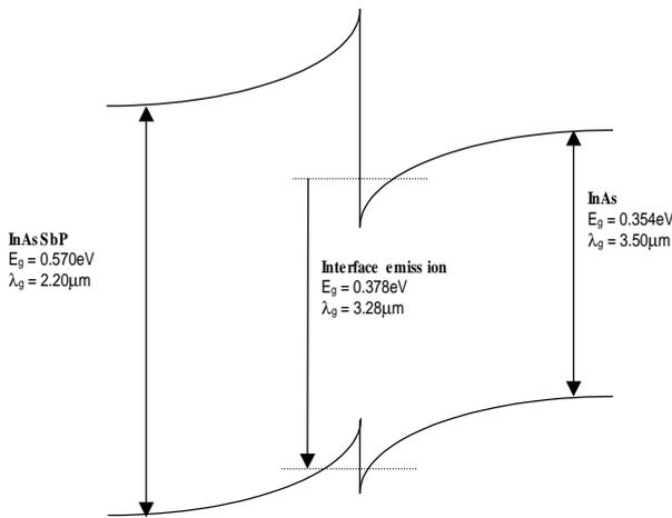
**Figure 7.** A schematic energy-band diagram of the heterojunction showing the type II interface transition observed in our LEDs at 3.28  $\mu\text{m}$  in the room-temperature electroluminescence spectrum.
